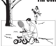
This unit has spinning mower blades. These blades can pick up and throw debris that could seriously injure a bystander. Be sure to clean up the area to be mowed BEFORE you start mowing.
